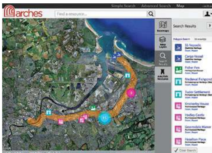
This screen shot of Arches depicts a user-defined polygon search for heritage resources in the area of a simulated construction project. Heritage resources within the polygon that would be impacted appear as icons. When many heritage assets are in close proximity in a map view, a cluster icon appears and displays the number of heritage assets that cluster represents. Image: © 2013 Google Map Data.
